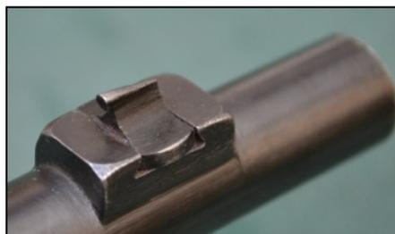
The No8 rearsight is a lovely little aperture rearsight purposely designed by BSA for the Martini rifles and provides target grade accuracy and maximises the rifle's capability. Although this is a sporting rifle, the sights' multiple apertures would have provided the shooter with both target and hunting capability.
