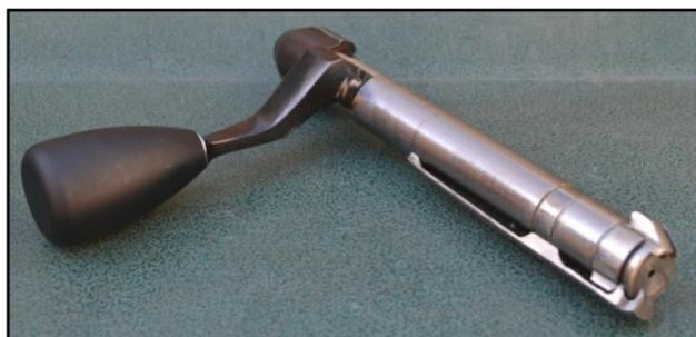
break the extractor and unlike the classic Mauser designs of WWII, the CZ bolt only has two locking lugs located in the bolt head. However whilst the bolt has lost its third safety lug it is apparent that when the bolt handle is fully depressed, the bolt handle is fully engaged in the receiver and should there be a catastrophic failure the bolt handle would act as a safety lug.
