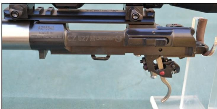
The bolt release/bolt stop is a different design to the large Mauser but the operating principle is identical. The 527 carbine safety catch is integral with the receiver and cannot be applied unless the bolt is cocked. Applying the safety catch disengages the cocking piece from the sear and locks the bolt.
