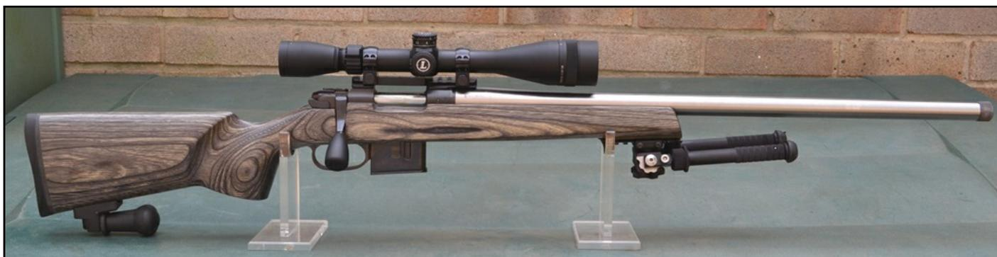
accurate rifle. This transformation has been largely due to the 6.5mm Grendel cartridge and at the time of updating this report, it has become a very popular round. Looking back, the rifle has seen a number of modifications to bring it up to this level and these include, new barrel, basix trigger, laminate stock, bedded action, tactical bolt knob, magazine catch extension, monopod, forend picatinny rail, Atlas bipod, Apex scope rail, Rechnagel rings and Leupold AR 6-18x44 scope.
