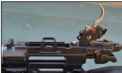
As a result I purchased a Basix after market trigger and found it to be far superior. The trigger is advertised as a "DIY" design, however you have to fit the new trigger into the current assembly and any foul-ups will make the rifle unsafe. Therefore I would recommend that this job is left to an Armourer/Gunsmith. The new trigger converts the set trigger function into a traditional single pull design which can be reduced to 1.0lb, making the rifle far more accurate and efficient to use.
