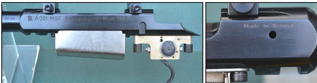
The front of the receiver is threaded to receive the barrel and either side of the receiver are the two largest flats measuring 18.5mm. These two ground surfaces match corresponding surfaces in the stock thereby provid-
