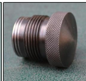
At the rear of the receiver is a large screw cap which secures the mainspring, its guide and the bolt. The screw cap is secured by a grub screw to prevent its unscrewing, however should the cap unscrew it can only rotate 2mm before engaging the rear of the stock, thereby preventing unscrewing any further.
