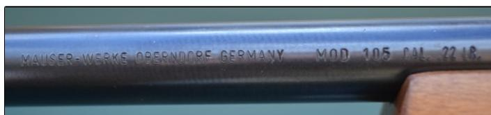
The receiver is stamped with the serial number and has the Mauser crest. The barrel is stamped with Mauser's title, model number and calibre. Blueing is good but lacks the quality and depth of the Mauser 201 but that is expected for the type of market this rifle is aimed at.
