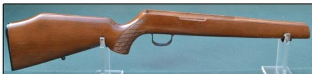
grip and simple sling swivels. Internally machining is good and the barrel and action fit well. The action is secured using a single main screw and the barrel does not float as it is designed to sit on the forend. The trigger guard is a simple press steel design, sits on a fascia plate and secures direct to the stock. Butt plate is a simple plastic affair that in this rifle, has taken an impact or two, whilst OK if I can find a new or serviceable plate, I will replacement it.
