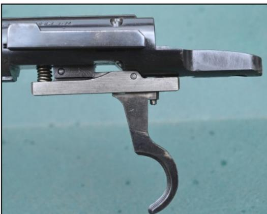
As with the K98, stripping the trigger is simplistic and for cleaning purposes the user should only need to remove the pin directly behind the trigger spring,
