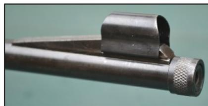
The foresight is a longitudinal blade and secures in a dovetail and is locked in place by a spring loaded stud. It has no adjustment, other than by changing blade sizes. The ramp is silver soldered in place, the front face of the ramp is serrated to minimise reflection and it is fitted with a fore sight protector
