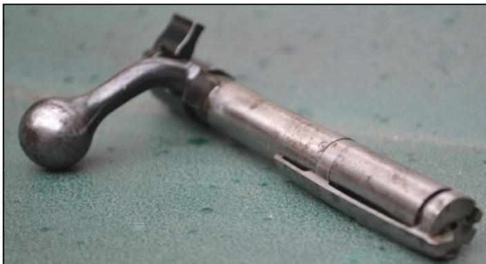
The bolt shroud contains the sear, firing pin, firing pin spring and safety and they function in exactly the same manner as the K98. With the safety lever sitting at the 9 o'clock position the rifle is ready to fire. Lifting the safety to the 12 o'clock, disengages the sear but permits the bolt to function, therefore allowing the operator to function the bolt, clear the chamber and empty the magazine. Rotating the safety to the 3 o'clock position, disengages the sear and locks the bolt.
