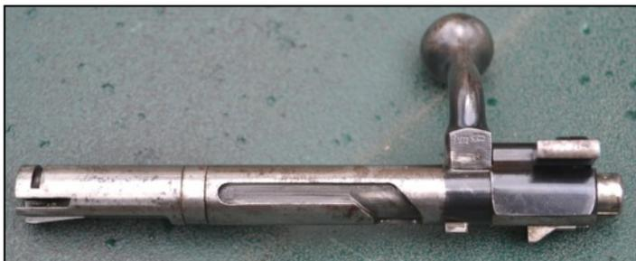
However unlike the K98 bolt, the locking lug is at the rear which assists in a smoother cycling action and the bolt stop engages in the recess machined in the centre of the bolt.
