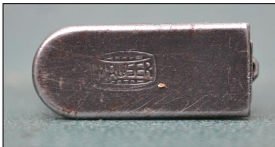
As .22 rimfire ammunition is what I would call “dirty” these magazines soak up all the wax and debris like a proverbial sponge and therefore the user should aim to give these magazines a good clean on an annual basis. Failure to do so will cause the platform to stick.
