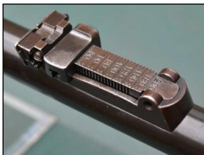
The rearsight is a ramp, with an unusual graduation - 30, 50, 80, 100, 125, 150, 180, 200 meters and utilises a slider for elevation adjustment.
