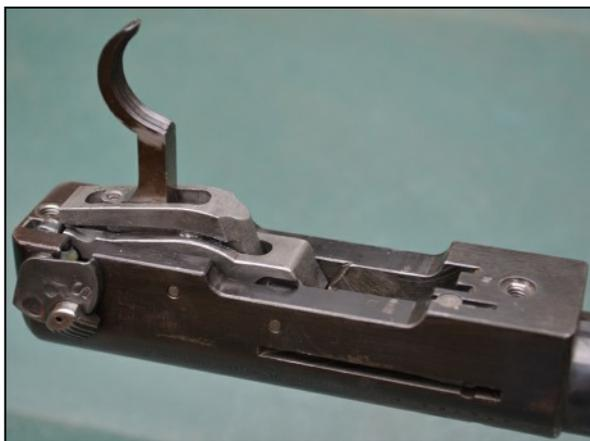
Trigger pressure is adjustable utilising a small screw at the rear of the trigger and on this particular rifle has a trigger pressure is 2.2lbs I have not attempted to adjust the trigger as access to the screws locking nut is difficult as it is shrouded by the lower assembly and may require a special tool. Whilst the trigger pressure is reasonable, the sear release is somewhat of a drag before the cocking piece is released.
