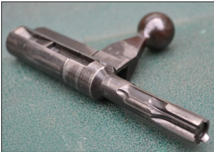
The long slender section is the bolt head and is integral with the bolt handle and contains the extractor claw and its spring. The rear section of the bolt assembly contains the cocking piece, firing pin, firing pin spring and is retained in the guide way by the rib directly behind the bolt handle.
