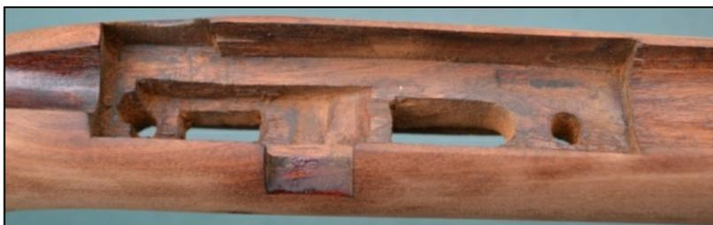
The stock is made from walnut and lacks any checkering, it is fitted with standard sling swivels, a plastic butt plate which is checkered and has the Mauser logo. Specific areas such as the barrel trough and magazine housing are machined but the receiver and relief for the trigger have been chiseled out by hand.
