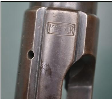
To manufacture this receiver would have taken a considerable number of machining operations, which by today standard would have made it very expensive, which is why the Mm410B which replaced it was a more simplistic design from a manufacturing standpoint.
