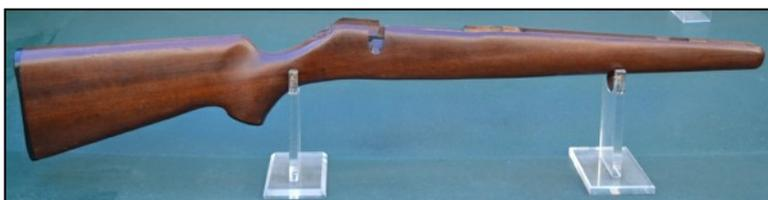
admirably. My particular stock had been well looked over the years and with the exception of the odd transit mark had weathered the years well. The stock had been modified to accept the screw for the rear tang and had been bedded with the old fibreglass bedding material utilised prior to the introduction of the more modern two pack epoxy resins we know today.
