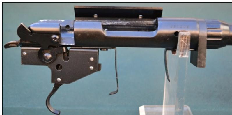
has a two gas escape ports, parallel to one another on either side of the receiver. Above the right gas port is the rifles serial number (152309) and behind this the rifles ejection port. The receiver walls at this point are fairly substantial at 0.28"(7.2mm) and generally remain so throughout the receivers length. Moving rearward is the bolt handle recess, which is the second/safety locking lug and the safety catch.
