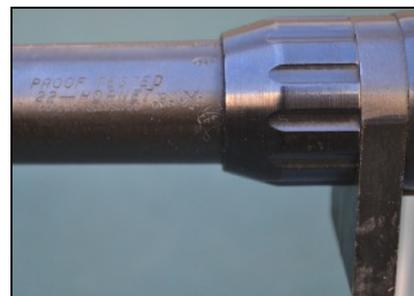
One odd observation which initially caused me concern is the chamber face has two steps which appear roughly machined, upon closer scrutiny this is to permit clearance for the extractor.
