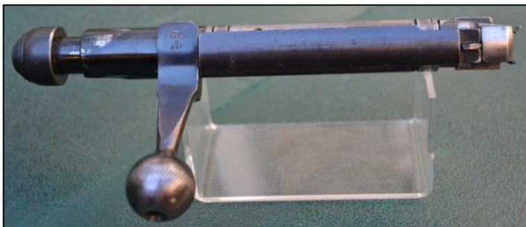
4 o'clock position on the bolt face is to allow the passage of the ejector. Whilst the locking lug provides the primary method of locking, the bolt handle clearly acts as a secondary point of locking and also as a safety lug should the main lug fail.
